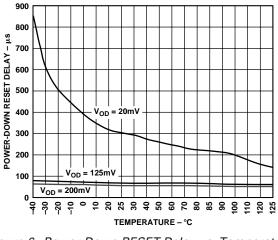
Figure 6. Power-Down RESET Delay vs. Temperature (ADM81\_L/M)
