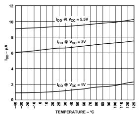
Figure 2. Supply Current vs. Temperature (ADM81\_R/S/T)
