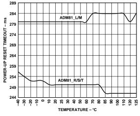
Figure 4. Power-Up Reset Timeout vs. Temperature
