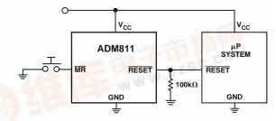
Figure 1. Typical Operating Circuit
