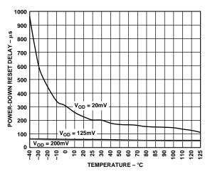
Figure 3. Power-Down RESET Delay vs. Temperature (ADM81\_R/S/T)
