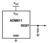
Figure 9. Ensuring a Valid  $\overline{RESET}$  Output Down to  $V_{CC} = 0 \ V$
