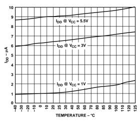
Figure 5. Supply Current vs. Temperature (ADM81\_L/M)
