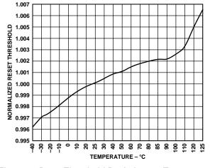
Figure 7. Reset Threshold Deviation vs. Temperature
