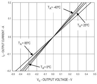
Figure 9. Typical Output Current vs Output Voltage
