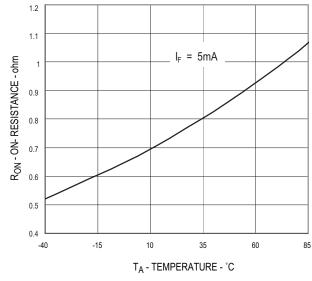
Figure 8. Typical on Resistance vs Temperature
