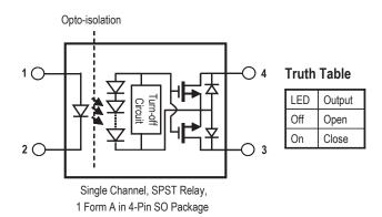
CAUTION: It is advised that normal static precautions be taken in handling and assembly of this component to prevent damage and/or degradation which may be induced by ESD.
