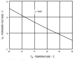
Figure 6. Typical Forward Voltage vs Temperature
