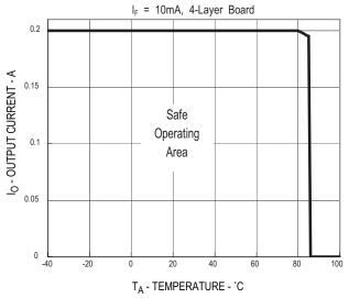
Figure 2. Maximum Output Current Rating vs Ambient Temperature (ASSR-1219-001E)
