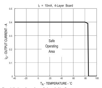
Figure 3. Maximum Output Current Rating vs Ambient Temperature (ASSR-1219-001E DC Connection)
