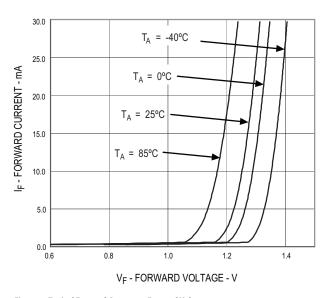
Figure 7. Typical Forward Current vs Forward Voltage
