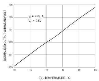
Figure 5. Normalized Output Withstand Voltage vs Temperature
