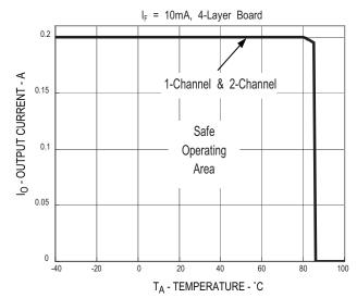
Figure 4. Maximum Output Current Rating vs Ambient Temperature (ASSR-1228-002E)
