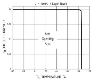
Figure 1. Maximum Output Current Rating vs Ambient Temperature (ASSR-1218-003E)
