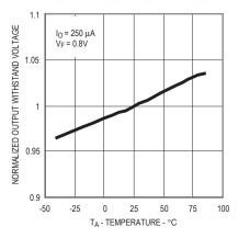
Figure 3. Normalized Typical Output Withstand Voltage vs. Temperature
