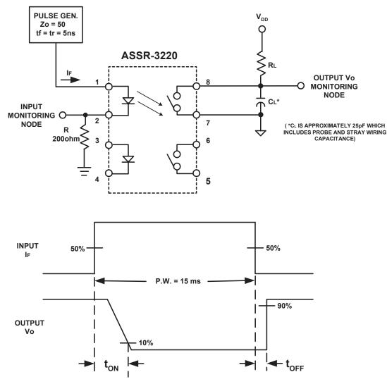
Figure. 13 Switching Test Circuit for TON, TOFF
