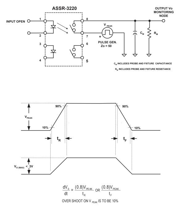
Figure. 14. Output Transient Rejection Test Circuit
