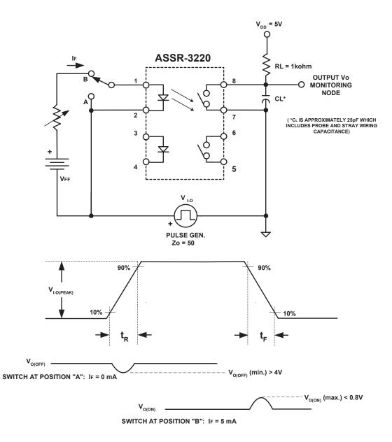
Figure 15. Input-Output Transient Rejection Test Circuit
