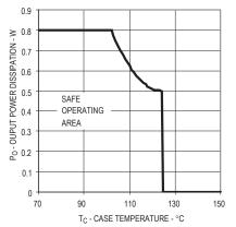
Figure 2. Output Power Derating vs Case Temperature
