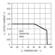
Figure 1. Maximum Average Output Current Rating vs
