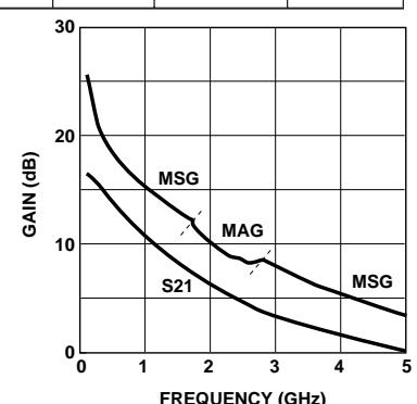
**AT-32011 Typical Scattering Parameters**, Common Emitter,  $Z_o = 50 \Omega$        $V_{CE} = 2.7 \text{ V}$ ,  $I_C = 20 \text{ mA}$
