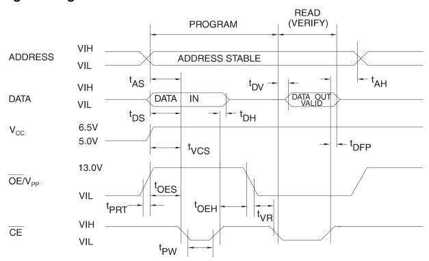
Notes: 1. The Input Timing Reference is 0.8V for  $V_{\rm IL}$  and 2.0V for  $V_{\rm IH}$ .
