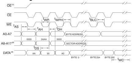
Notes: 1.  $\overline{OE}$  must be high when  $\overline{WE}$  and  $\overline{CE}$  are both low.
