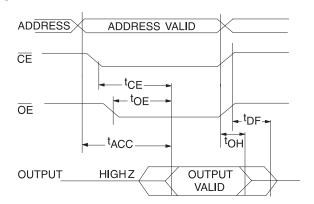
Notes: 1.  $\overline{\text{CE}}$  may be delayed up to  $t_{\text{ACC}}$  -  $t_{\text{CE}}$  after the address transition without impact on  $t_{\text{ACC}}$ .
