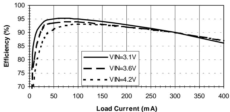
Note: 1.  $L = 10 \mu\text{H}$ ,  $\text{ESR} = 0.2 \Omega$ ,  $c = 22 \mu\text{F}$ , @ $\text{ESR} = 0.1 \Omega$
