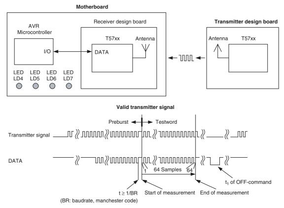
The AVR microcontroller continuously measures the time between two signal edges (= 1 sample). If the time t  $\geq$  1/baud rate, the following 64 samples will be stored in the RAM of the microcontroller (start of measurement/end of measurement, see Figure 5-2 on page 9). Then, the RF receiver will be set back to polling mode by the microcontroller pulling pin DATA to '0' for a time t<sub>1</sub>. The timing limits of 1/baud rate are programmable in the RF Design Kit software.
