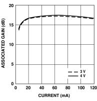
Figure 7. Associated Gain vs. Current  $(I_d)$  and Voltage  $(V_D)$  at 2 GHz. $^{[1,2]}$
