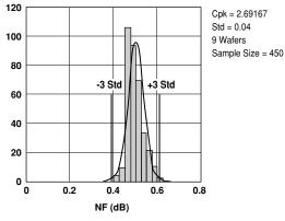
**Figure 3. NF @ 2 GHz, 4 V, 60 mA.** LSL=0.1, Nominal=0.47, USL=0.8
