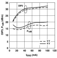
Figure 9. OIP3 and  $P_{1dB}$  vs.  $I_{DS}$  and  $V_{DS}$  Tuned for NF @ 4 V, 60 mA at 900 MHz.  $\left[1,2\right]$
