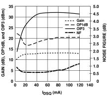
Figure 16. NF, Gain, OP1dB and OIP3 vs.  $I_{DS}$  at 4 V and 3.9 GHz Tuned for Noise Figure.<sup>[1]</sup>
