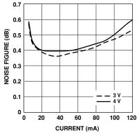
Figure 11. Noise Figure vs. Current ( $I_d$ ) and Voltage ( $V_{DS}$ ) at 900 MHz.  $^{[1,2]}$
