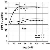
Figure 6. OIP3 and  $P_{\rm 1dB}$  vs.  $I_{\rm DS}$  and  $V_{\rm DS}$  Tuned for NF @ 4 V, 60 mA at 2 GHz, [1,2]
