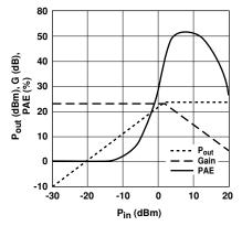
Figure 20. Swept Power Tuned for Power at 2 GHz,  $V_{\rm DS}$  = 4 V,  $I_{\rm DSQ}$  = 120 mA.
