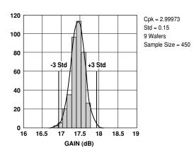
**Figure 4. Gain @ 2 GHz, 4 V, 60 mA.** LSL=16.0, Nominal=17.5, USL=19.0
