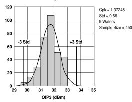
**Figure 2. OIP3 @ 2 GHz, 4 V, 60 mA.** LSL=29.0, Nominal=31.8, USL=35.0
