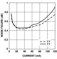
Figure 8. Noise Figure vs. Current  $(I_d)$  and Voltage  $(V_{DS})$  at 2 GHz.  $^{[1,2]}$
