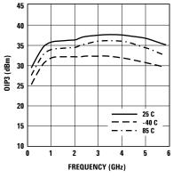
Figure 16. OIP3 vs. Frequency and Temp Tuned for Max OIP3 and Fmin at 3V, 60 mA.
