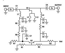
Figure 2. Typical ATF-54143 LNA with Active Biasing.
