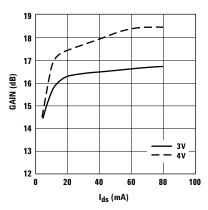
Figure 8. Gain vs.  $I_{ds}$  and  $V_{ds}$  Tuned for Max 0IP3 and Fmin at 2 GHz.
