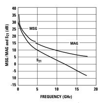
Figure 20. MSG/MAG and  $\mid$   $S_{21}\mid^2$  vs. Frequency at 3V, 60 mA.
