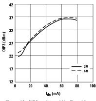
Figure 10. OIP3 vs.  $I_{ds}$  and  $V_{ds}$  Tuned for Max OIP3 and Fmin at 2 GHz.
