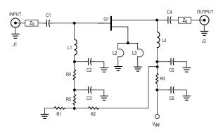
Figure 1. Typical ATF-54143 LNA with Passive Biasing.
