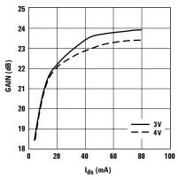
Figure 9. Gain vs.  $I_{ds}$  and  $V_{ds}$  Tuned for Max 0IP3 and Fmin at 900 MHz.
