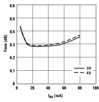
Figure 7. Fmin vs.  $I_{ds}$  and  $V_{ds}$  Tuned for Max 0IP3 and Min NF at 900 MHz.
