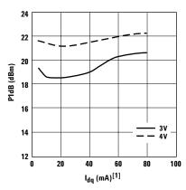
Figure 12. P1dB vs.  $I_{dq}$  and  $V_{ds}$  Tuned for Max 0IP3 and Fmin at 2 GHz.
