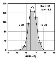
Figure 3. Gain @ 2 GHz, 3 V, 60 mA. USL = 18.5, LSL = 15, Nominal = 16.6
