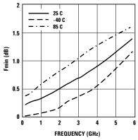
Figure 15. Fmin<sup>[2]</sup> vs. Frequency and Temp Tuned for Max OIP3 and Fmin at 3V, 60 mA.
