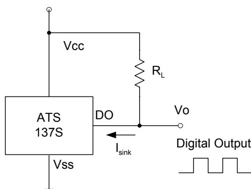
Fig.2 Application circuit
