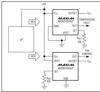
Figure 6. Low-Power, High-Reliability, Fail-Safe Temperature Monitor
