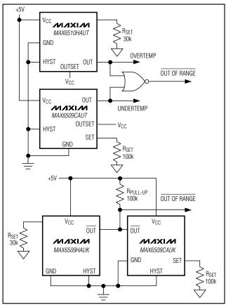
Figure 5. Temperature-Window Detector
