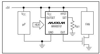
Figure 3. Overtemperature Fan Control
