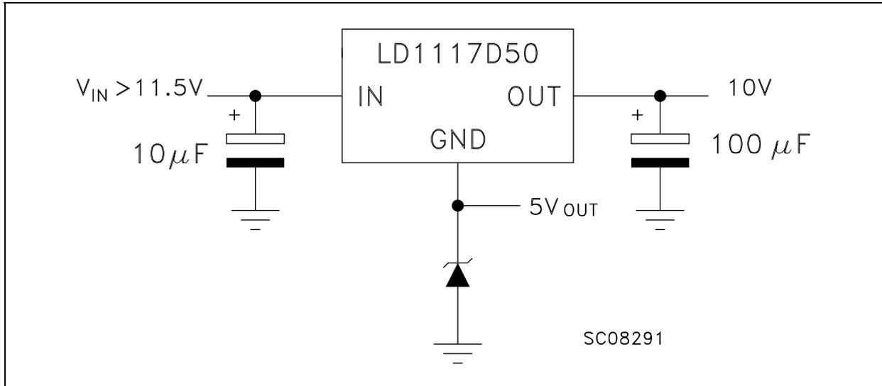
Figure 5 : Battery Backed-up Regulated Supply
