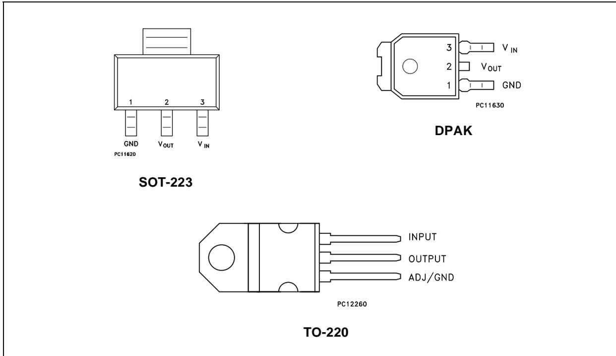
NOTE: The TAB is connected to the V<sub>OUT</sub>.
