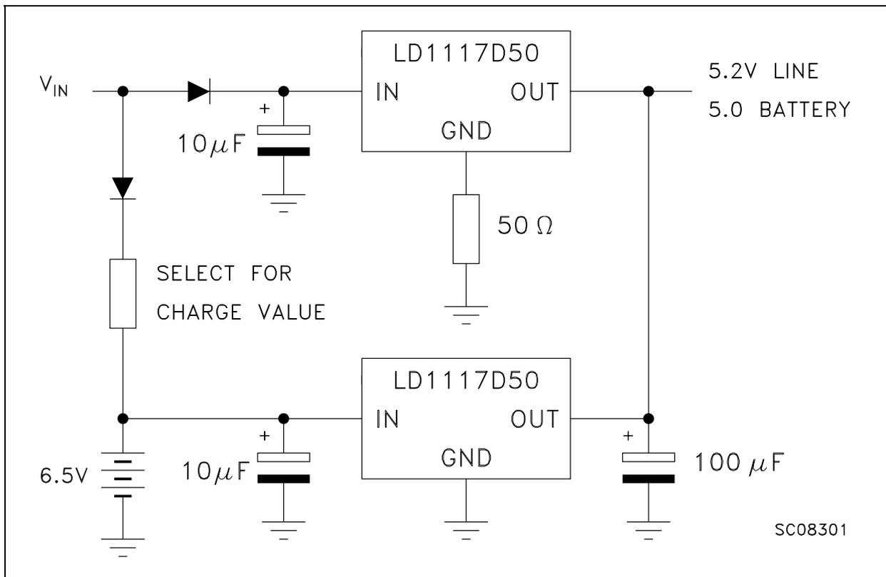
Figure 6 : Post-Regulated Dual Supply
