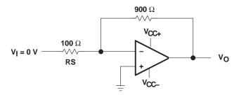
Figure 2. Noise-Test Circuit
