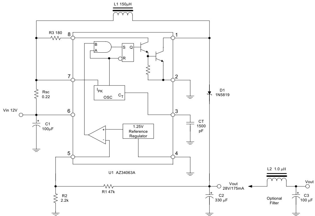
Figure 10. Step-Up Converter (Note 5)
