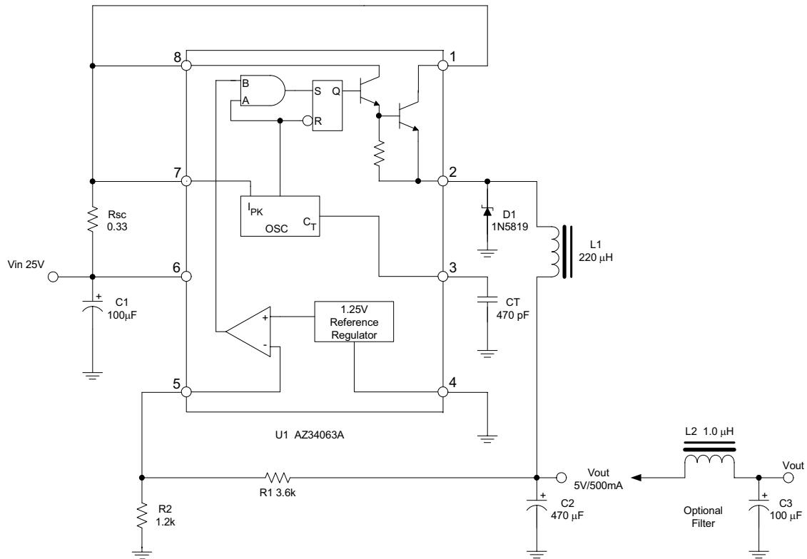
Figure 11. Step-Down converter (Note 6)
