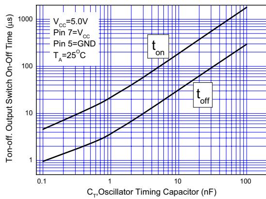
Figure 4. Output Switch On-Off Time vs.
