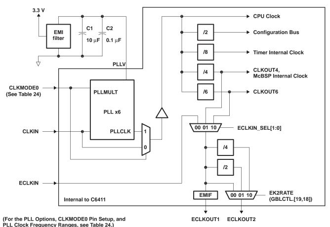
NOTES: A. Place all PLL external components (C1, C2, and the EMI Filter) as close to the C6000™ DSP device as possible. For the best performance, TI recommends that all the PLL external components be on a single side of the board without jumpers, switches, or
