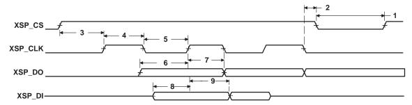
Figure 50. PCI Serial EEPROM Interface Timing
