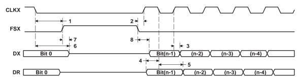
Figure 53. McBSP Timing as SPI Master or Slave: CLKSTP = 10b, CLKXP = 0
