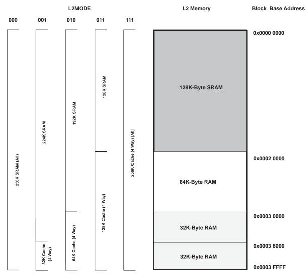
Figure 2. TMS320C6411 L2 Architecture Memory Configuration
