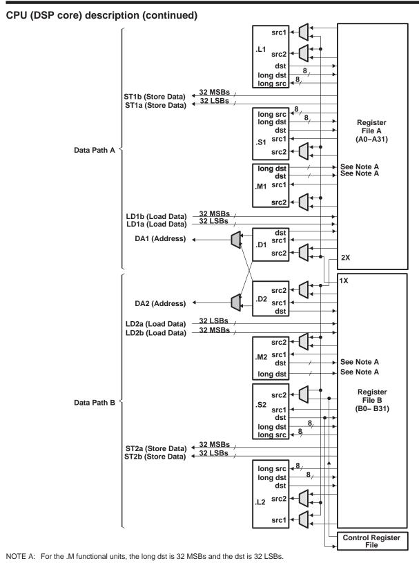
Figure 1. TMS320C64x™ CPU (DSP Core) Data Paths
