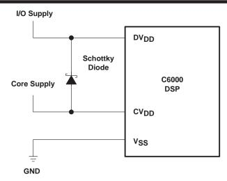
Figure 11. Schottky Diode Diagram
