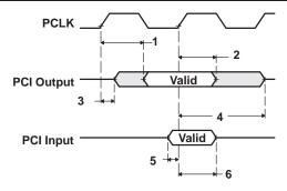
Figure 49. PCI Intput/Output Timing
