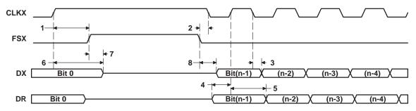
Figure 55. McBSP Timing as SPI Master or Slave: CLKSTP = 10b, CLKXP = 1
