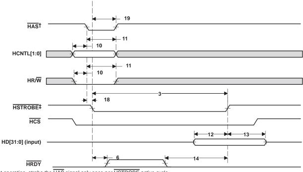
† For correct operation, strobe the HAS signal only once per HSTROBE active cycle.
