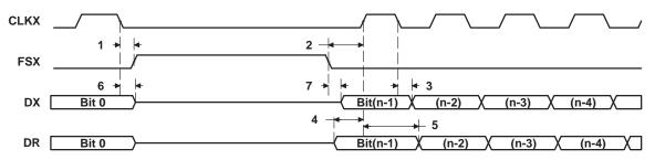
Figure 54. McBSP Timing as SPI Master or Slave: CLKSTP = 11b, CLKXP = 0
