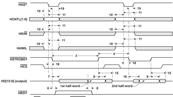
Figure 40. HPI16 Read Timing (HAS Used)
