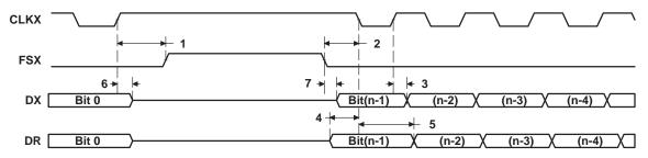
Figure 56. McBSP Timing as SPI Master or Slave: CLKSTP = 11b, CLKXP = 1
