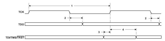
Figure 59. JTAG Test-Port Timing
