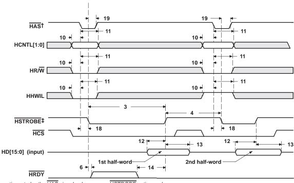
Figure 42. HPI16 Write Timing (HAS Used)
