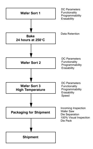
Figure 1. AMD KGD Product Test Flow
