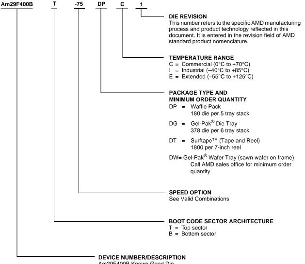
Am29F400B Known Good Die 4 Megabit (512 K x 8-Bit/256 K x 16-Bit) CMOS Flash Memory—Die Revision 1 5.0 Volt-only Program and Erase
