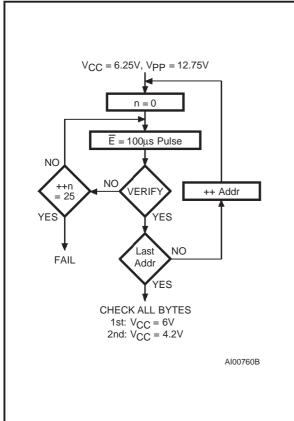
Figure 8. On-Board Programming Flowchart
