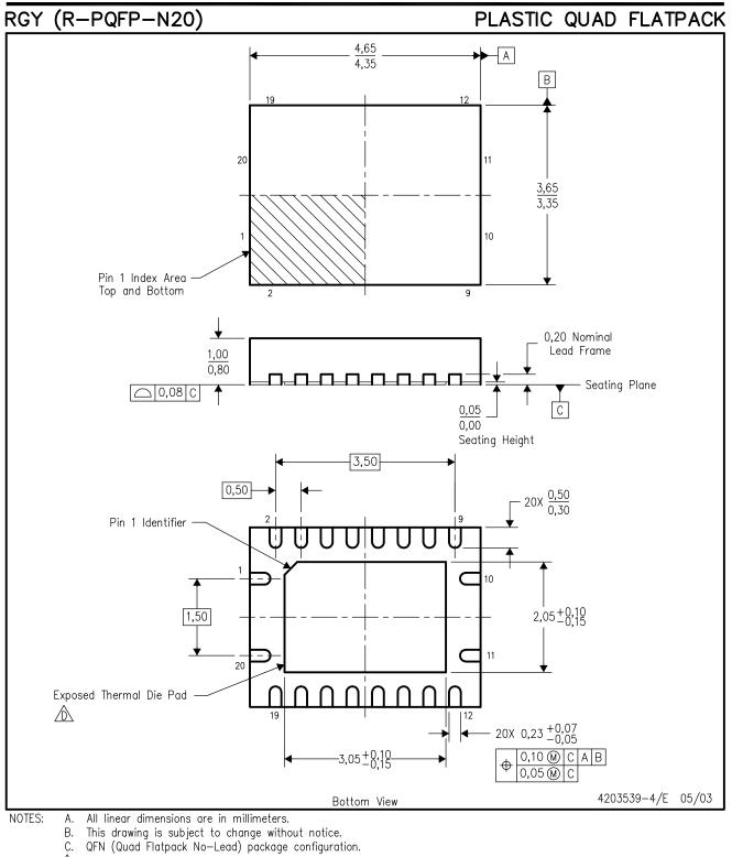
The package thermal performance may be enhanced by bonding the thermal die pad to an external thermal plane. This pad is electrically and thermally connected to the backside of the die and possibly selected ground leads.
