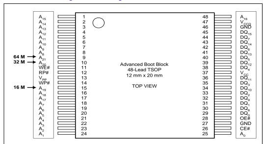
Figure 2. 48-Lead TSOP Package for x16 Configurations
