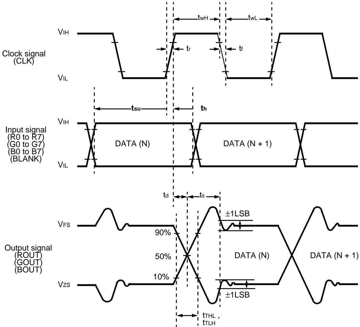
**Note:** R0 to R7, G0 to G7, B0 to B7 are read on the rising edge of the clock.
