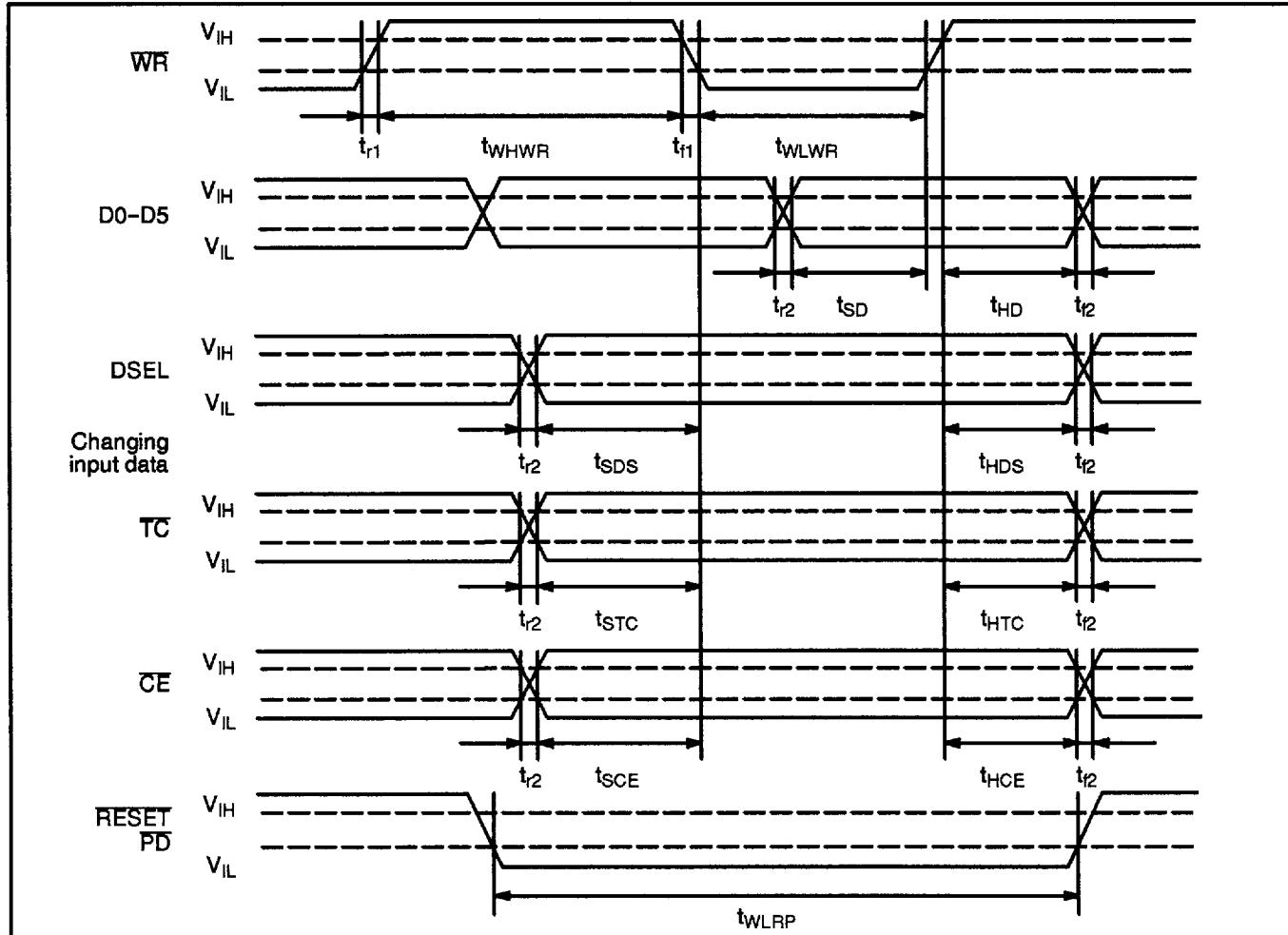
**Figure 4. Timing Diagram ( $CE = L$ )**
