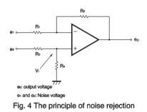
With the BA3121, the elimination level of the noise is expressed as: CMMR = 20log  $(e_0/e_i)$   $(e_i = e_1 = e_2)$ Therefore, CMRR  $\ge$  41dB can be guaranteed.
