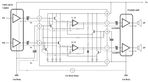
Fig. 3 Flow of noise in car-audio systems
