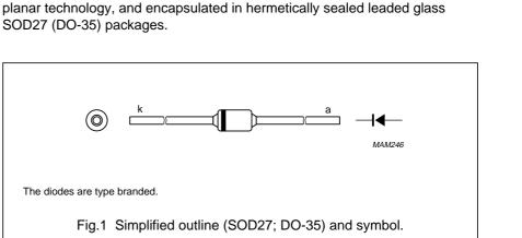
The BA316, BA317, BA318 are high-speed switching diodes fabricated in
