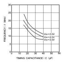
Fig. 7 Frequency vs. timing capacitor capacitance
