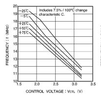
Fig. 4 Frequency vs. control voltage temperature
