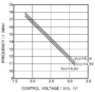
Fig. 5 Frequency vs. control voltage temperature
