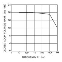
Fig. 6 Closed loop voltage gain vs. frequency (reversing amplifier)
