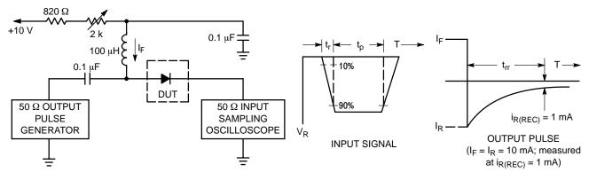
Notes: 1. A 2.0 k $\Omega$  variable resistor adjusted for a Forward Current (I<sub>F</sub>) of 10 mA. 2. Input pulse is adjusted so I<sub>R(peak)</sub> is equal to 10 mA.
