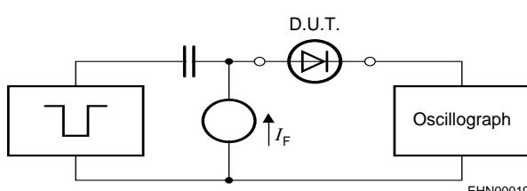
Pulse generator:  $t_p = 10\mu\text{s}$ ,  $D = 0.05$ ,
