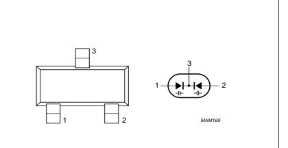
Fig.1 Simplified outline (SOT23), pin configuration and symbol.
