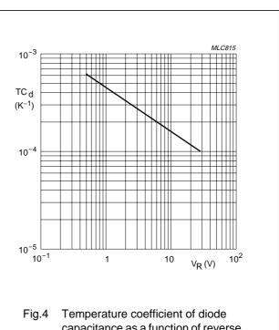
capacitance as a function of reverse voltage; typical values.
