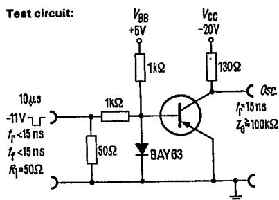
Switching times for transistors
