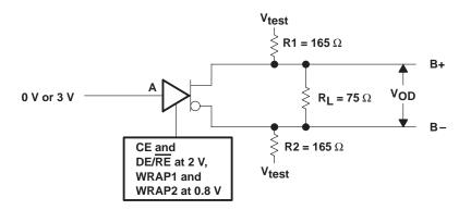
Figure 1. Driver V<sub>OD</sub> Test Circuit
