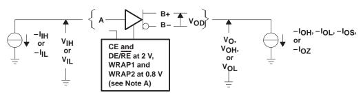
NOTE A: For the I<sub>OZ</sub> test, the CE input is at 0.8 V.
