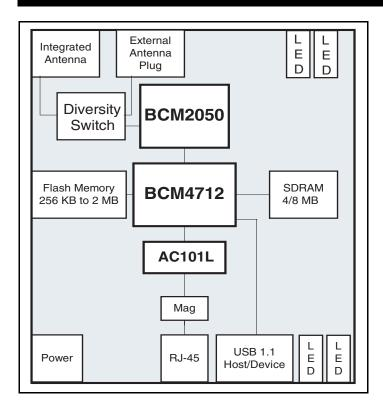
The BCM94712 reference design is a fully integrated access point that combines small size, rich features, and advanced components into the most cost effective access point in the AirForce™ product family and the wireless LAN industry. As small as a credit card, this AP incorporates an integrated antenna, an integrated IEEE 802.11g MAC/baseband, and USB host/device functions enabling manufacturers to build highly functional and low-cost Wi-Fi® access points.
