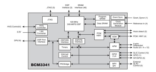
The **BCM3341** offers the industry a highly integrated, cost effective approach to developing PacketCable™ or DSL VoIP solutions for the delivery of primary or secondary line telephony. The **BCM3341** provides a seamless interface with multiple Broadcom cable, DSL and IP phone products. This includes the BCM3348, BCM3360 and BCM3370 cable modem IC solutions, the BCM6350, BCM6352, BCM6345 DSL IC solutions, and the BCM1101 SMTA and IP phone solutions.
