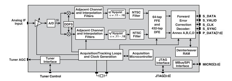
The Broadcom BCM3510 is a VSB/QAM digital receiver, compatible with both North American digital cable television and digital terrestrial broadcast television standards. It is capable of receiving all standard-definition and high-definition digital television formats (SDTV/HDTV).
