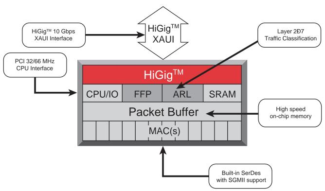
The **BCM5690** network switch is a scalable, modular chip solution with 12 ports. Each of these flexible ports supports Gigabit Ethernet or 10/100 Mbps Ethernet. Additionally, the **BCM5690** supports both copper and fiber physical interfaces. The **BCM5690** has a fully integrated SerDes functionality consisting of a 10 Gbps XAUI HiGig Port, Gigabit Ethernet or a SGMII PHY interface.
