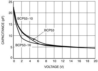
Figure 11. Output Capacitance
