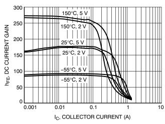
Figure 4. DC Current Gain vs. Collector Current (BCP53-16)
