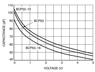
Figure 10. Input Capacitance
