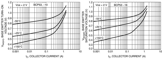
Figure 7. BCP53, -10 Base Emitter Turn-On Voltage vs. Collector Current V<sub>BE(on)</sub>
