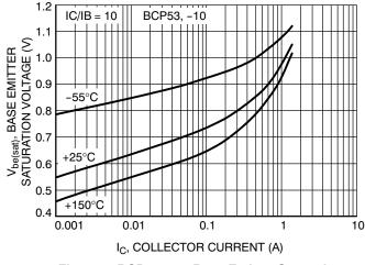
Figure 5. BCP53, -10 Base Emitter Saturation Voltage vs. Collector Current
