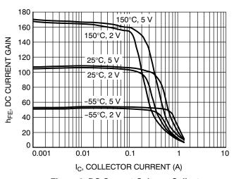
Figure 3. DC Current Gain vs. Collector Current (BCP53-10)
