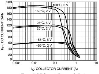
Figure 2. DC Current Gain vs. Collector Current (BCP53)
