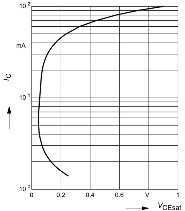
**Input on Voltage  $V_{i(on)} = f(I_C)$**
