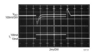
This photo shows transient response in constant switching mode with a 10mA to 100mA stepped load. Output ripple at the switching frequency can be reduced considerably by adding a  $10\mu F$  ceramic capacitor in parallel with the  $100\mu F$  tantalum.
