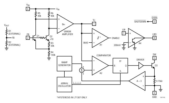
Figure 2. LT1307/LT1307B Block Diagram
