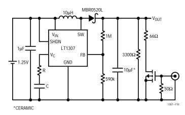
Figure 10. Boost Converter with Simulated Load
