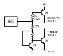
Figure 13. Shutdown Circuit
