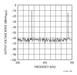
Figure 9. LT1307B at 5mA Load Shows No Audio Components or Sidebands About Switching Frequency, 333kHz Fundamental Amplitude is -10dBmV, or 316µV<sub>RMS</sub>
