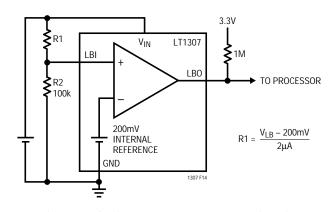
Figure 14. Setting Low-Battery Detector Trip Point
