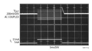
Figure 11a. V<sub>C</sub> Pin Left Unconnected. Output Ripple Voltage is 300mV<sub>P-P</sub> Under Load
