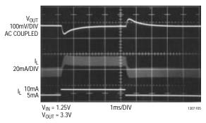
Figure 5. Increasing L to 100 $\mu$ H, Along with R<sub>C</sub> = 36k, C<sub>C</sub> = 20nF and C<sub>OUT</sub> = 10 $\mu$ F, Low Noise Performance of LT1307B Can Be Realized at Light Loads of 5mA to 10mA
