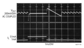
Figure 11e. A 100k/680pF RC Provides Optimum Settling Time with No Ringing
