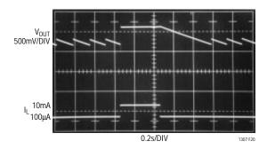
This photo details output voltage as the circuit is switched between the two modes. Load current is 100µA in Burst Mode operation; 10mA in constant switching mode.
