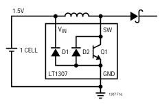
Figure 16. LT1307 Showing Internal Substrate Diodes D1 and D2. In Normal Operation Diodes are Reverse-Biased
