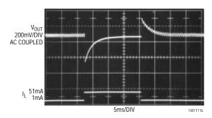
Figure 11b. Inclusion of a 100k/22nF Series RC on  $V_{\mathbb{C}}$  Pin Results in Overdamped Stable Response
