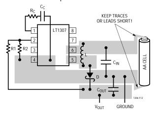
Figure 12. Recommended Component Placement. Traces Carrying High Current Are Direct. Trace Area at FB Pin and  $V_{\mathbb{C}}$  Pin is Kept Low. Lead Length to Battery Should Be Kept Short
