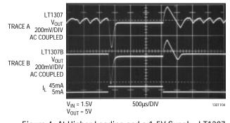
Figure 4. At Higher Loading and a 1.5V Supply, LT1307 Again Exhibits Burst Mode Operation Ripple at 5mA Load, LT1307B Does Not
