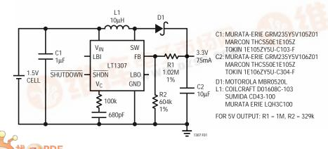
Figure 1. Single Cell to 3.3V Boost Converter
