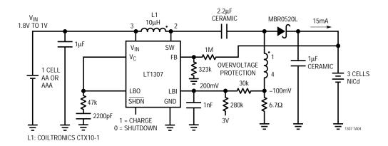
Single Cell Powered Constant Current LED Driver
