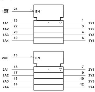
logic diagram (positive logic) 24 1<mark>OE</mark> 23 1 1Y1 1A1 22 3 1Y2 1A2 20 4 1A3 -1Y3 19 6 1A4 -— 1Y4 13 2<mark>0E</mark> 18 7 2Y1 2A1 17 9 2A2 2Y2 10 15
