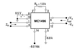
**NOTE:** Shielding of input and output leads may be needed to properly perform these tests.
