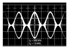
Figure 3. Amplitude Modulation Output Waveform
