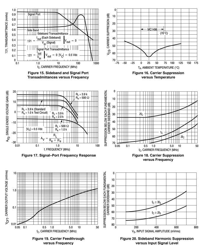
Typical characteristics were obtained with circuit shown in Figure 5, f<sub>C</sub> = 500 kHz (sine wave),  $V_C = 60 \text{ mVrms}$ , f<sub>S</sub> = 1.0 kHz,  $V_S = 300 \text{ mVrms}$ , T<sub>A</sub> = 25°C, unless otherwise noted.
