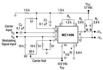
Figure 5. Carrier Rejection and Suppression
