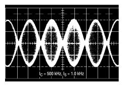
Figure 1. Suppressed Carrier Output Waveform
