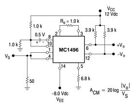
Figure 9. Common Mode Gain
