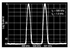
Figure 2. Suppressed Carrier Spectrum
