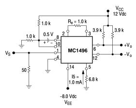
Figure 10. Signal Gain and Output Swing
