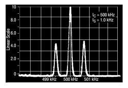
Figure 4. Amplitude–Modulation Spectrum
