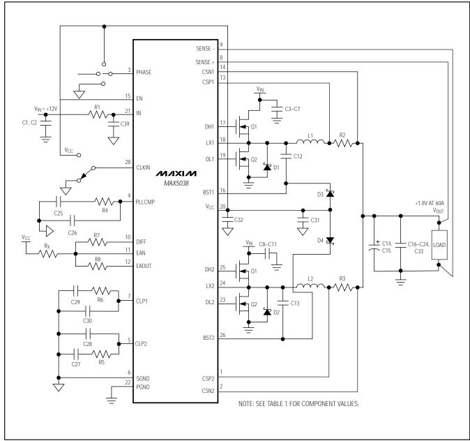
Figure 1. MAX5038 Typical Application Circuit, V<sub>IN</sub> = +12V
