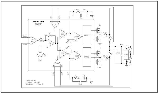
Figure 3b. MAX5041 Control Loop
