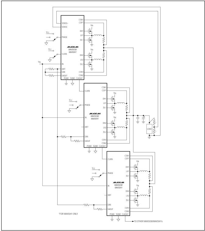
Figure 6. Parallel Configuration of Multiple MAX5038/MAX5041s
