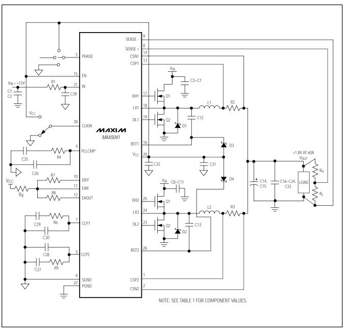
Figure 2. MAX5041 Typical Application Circuit, V<sub>IN</sub> = +12V
