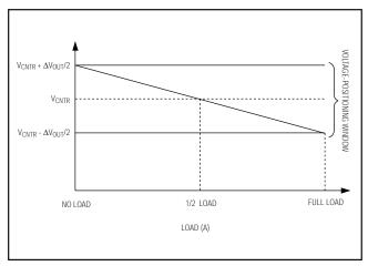
Figure 5. Defining the Voltage-Positioning Window
