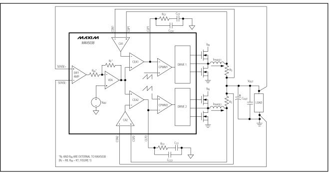
Figure 3a. MAX5038 Control Loop
