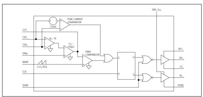
Figure 4. Phase Circuit (Phase 1/Phase 2)
