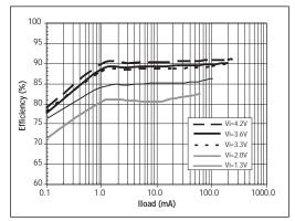
Figure 7. SP6641AEK-5.0 Efficiency Vs Load Current
