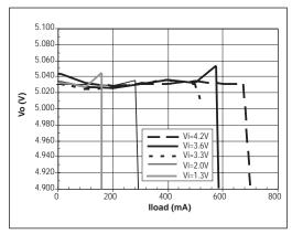
Figure 10. SP6641BEK-5.0 Line/Load Rejection Vs Load Current
