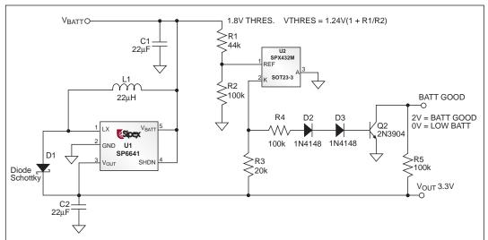
Figure 17 SP6641A 2 3V with Low Rattery Detection
