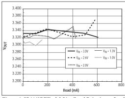
Figure 6. SP6641BEK - 3.3 Line/Load Rejection vs Load Current
