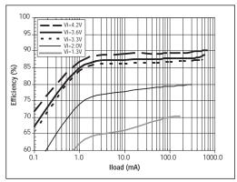
Figure 8. SP6641BEK-5.0 Efficiency Vs Load Current
