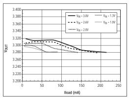
Figure 5. SP6641AEK - 3.3 Line/Load Rejection vs Load Current
