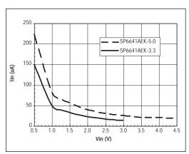
Figure 11. SP6641AEK-3.3 & SP6641AEK-5.0 No Load Battery Current
