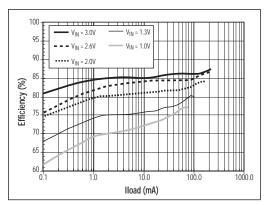
Figure 3. SP6641AEK - 3.3 Efficiency vs Load Current
