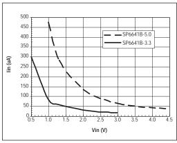
Figure 12. SP6641BEK-3.3 & SP6641AEK-5.0 No Load Battery Current
