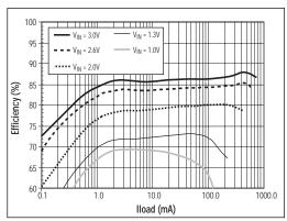
Figure 4. SP6641BEK - 3.3 Efficiency vs Load Current
