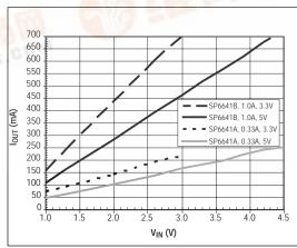
Figure 2. Maximum Load Current in Operation
