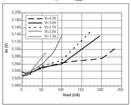
Figure 9. SP6641AEK-5.0 Line/Load Rejection Vs Load Current
