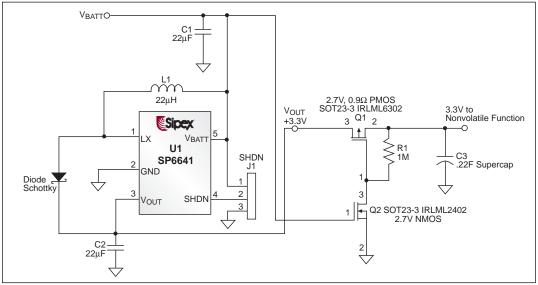
Figure 16. SP6641A 3.3V with SuperCap Switch
