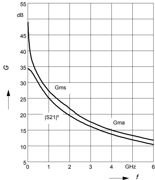
**Power gain  $G_{ma}, G_{ms} = f(V_{CE})$**
