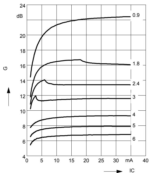
**Power gain  $G_{ma}$ ,  $G_{ms} = f(V_{CE})$**
