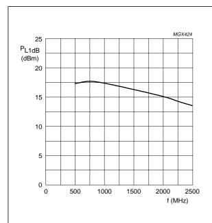
Fig.7 Load power as a function of frequency; typical values.
