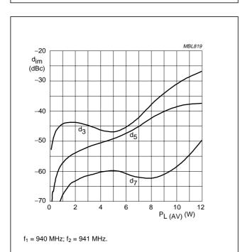
Fig.8 Two tone intermodulation distortion as a function of average load power; typical values.
