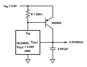
FIGURE 5. PRECISION 2.5V 50mA REFERENCE
