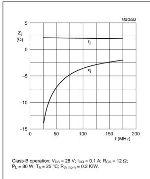
Fig.13 Input impedance as a function of frequency (series components), typical values.
