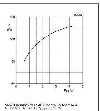
Fig.10 Load power as a function of input power,
