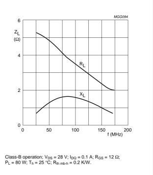
Fig.14 Load impedance as a function of frequency (series components), typical values.
