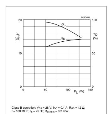
Fig.9 Power gain and efficiency as functions of load power, typical values.
