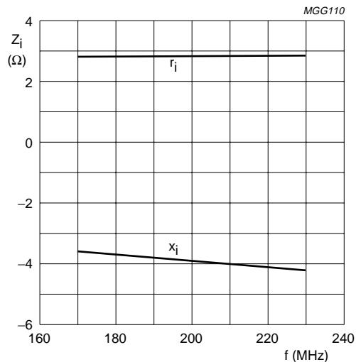
Class-A operation;  $V_{DS} = 28$  V;  $I_D = 3$  A;  $P_L = 30$  W;  $T_h = 70$  °C.
