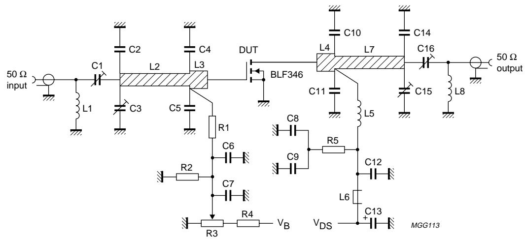
Fig.10 Test circuit for class-A operation at  $f = 225$  MHz.
