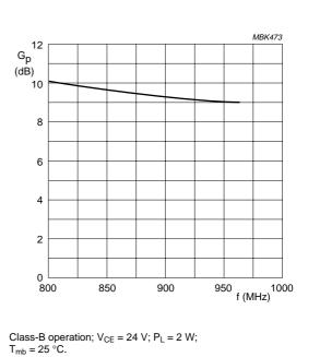
Fig.12 Power gain as a function of frequency, typical values.
