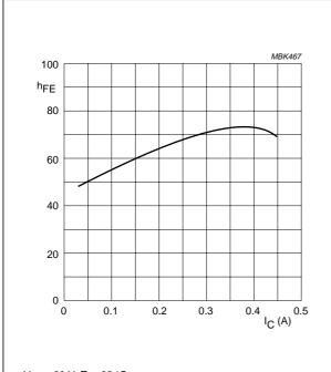
$V_{CE}$  = 20 V;  $T_{j}$  = 25  $^{\circ}C.$
