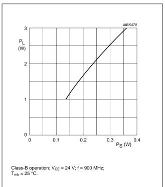
Fig.6 Load power as a function of drive power, typical values.
